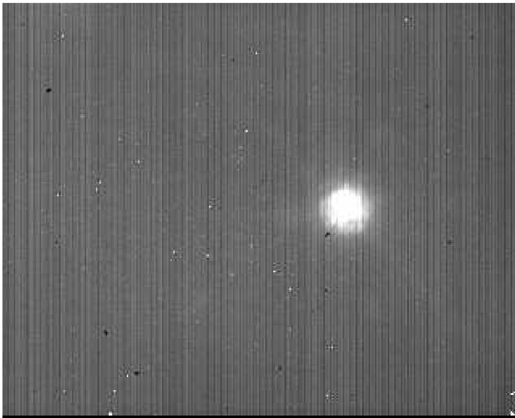
Figure 3.5 Raw Clio image of \epsilon Eri from nod position 2. Note the strong column striping from the detector, and other artifacts.
