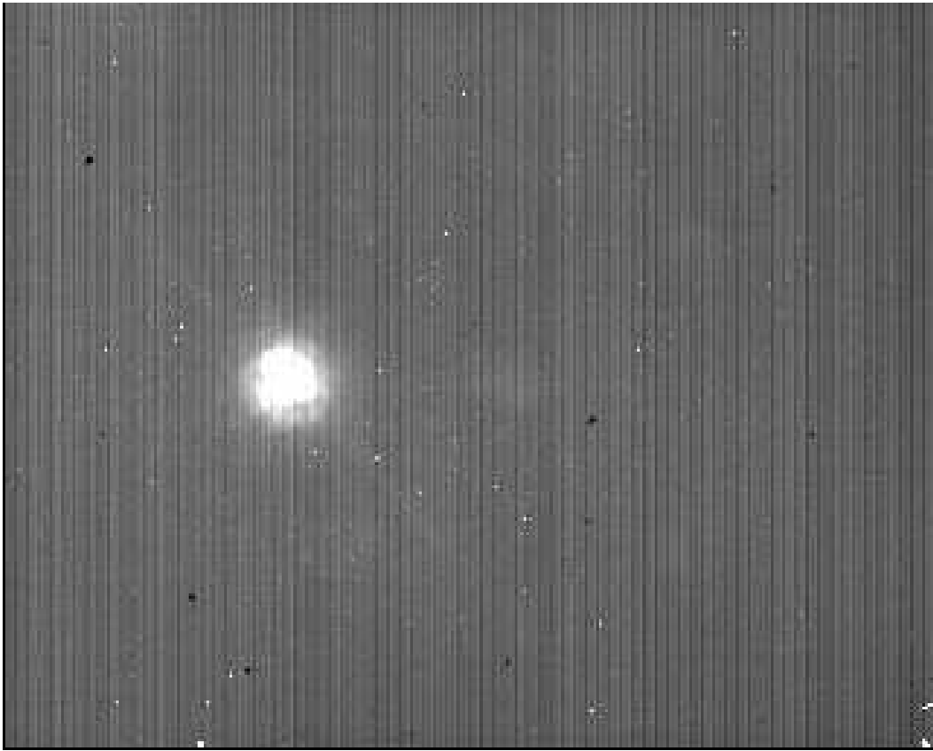
Figure A.1 Raw Clío image of \epsilon Eri from nod position 1. Note the strong column striping from the detector, and other artifacts.
